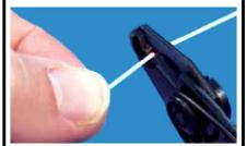
Check fiber for integrity by bending the stripped end of the fiber slightly.
